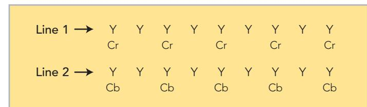
4:2:0 provides equal colour resolution vertically and horizontally if using square pixels
